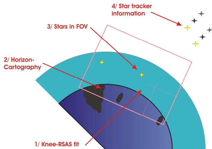
Figure 1 The attitude registration in limb observation mode is performed by the combination of the star tracker information, the position of stars in FOV and geographic features.
