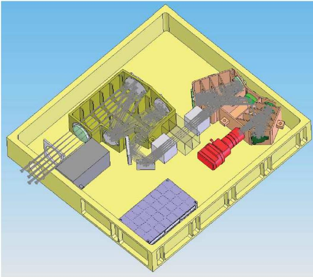
Figure 4: Conceptual design of the ALTIUS visible channel. Notice the neutral filter mechanism after the aperture in order to perform solar occultation measurements.
