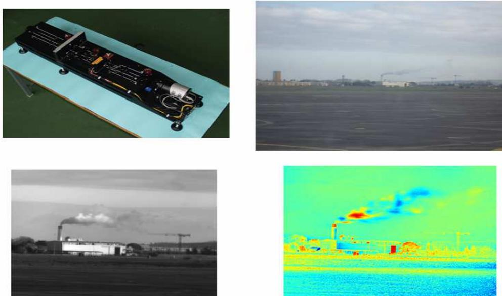
Figure 3 Top: ALTIUS visible breadboard (left); handheld camera picture of the observed scene (right). Bottom: snapshot at 645 nm (left) . Differential measurement in the NO<sub>2</sub> band (right).
